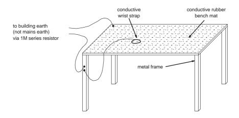
Figure 2.1 Typical Antistatic Bench Setup
